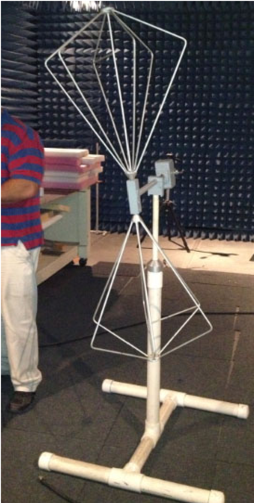
Radiated RF Emission sensed by Biconical Antenna Our unit in the chamber
